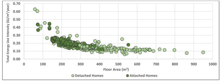
Figure 18: Total Energy Use Intensity by Floor Area
