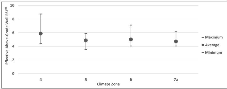
Figure 5: Attached Homes - Average Above-Grade Wall RSI<sup>eff</sup> by Climate Zone
