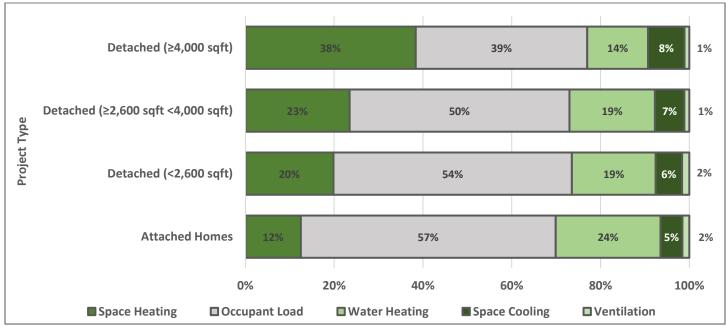
Figure 13: Average Load Distribution of Annual Energy Consumption by Floor Area
