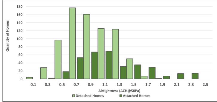
Figure 17: Distribution of Airtightness by ACH@50
