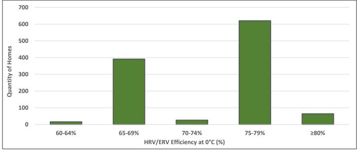
Figure 10: HRV/ERV Efficiency at 0°C
