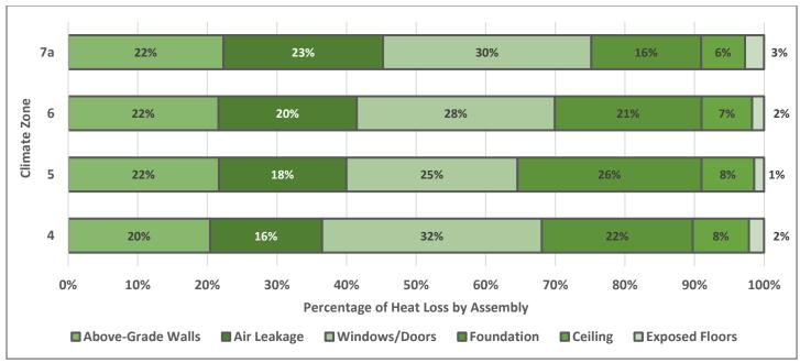
Figure 16: Attached Homes – Assembly Distribution of Whole Home Heat Loss by Climate Zone
