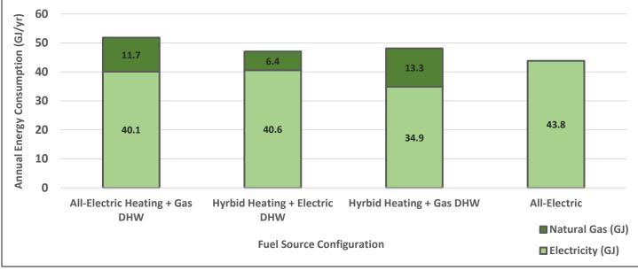
Figure 11: Fuel Source Consumption Comparison by System Configuration
