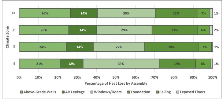
Figure 15: Detached Homes – Assembly Distribution of Whole Home Heat Loss by Climate Zone
