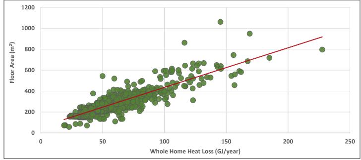
Figure 14: Whole Home Heat Loss by Floor Area
